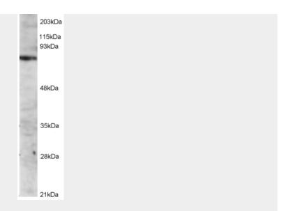
AF1575a staining (2  $\mu$ g/ml) of Jurkat lysate (RIPA buffer, 1.4E+05 cells per lane). Primary incubated for 12 hour. Detected by western blot using chemiluminescence.
